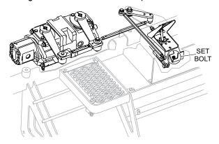
Figure 28. Trowel Speed Control (Set Bolt Location)
